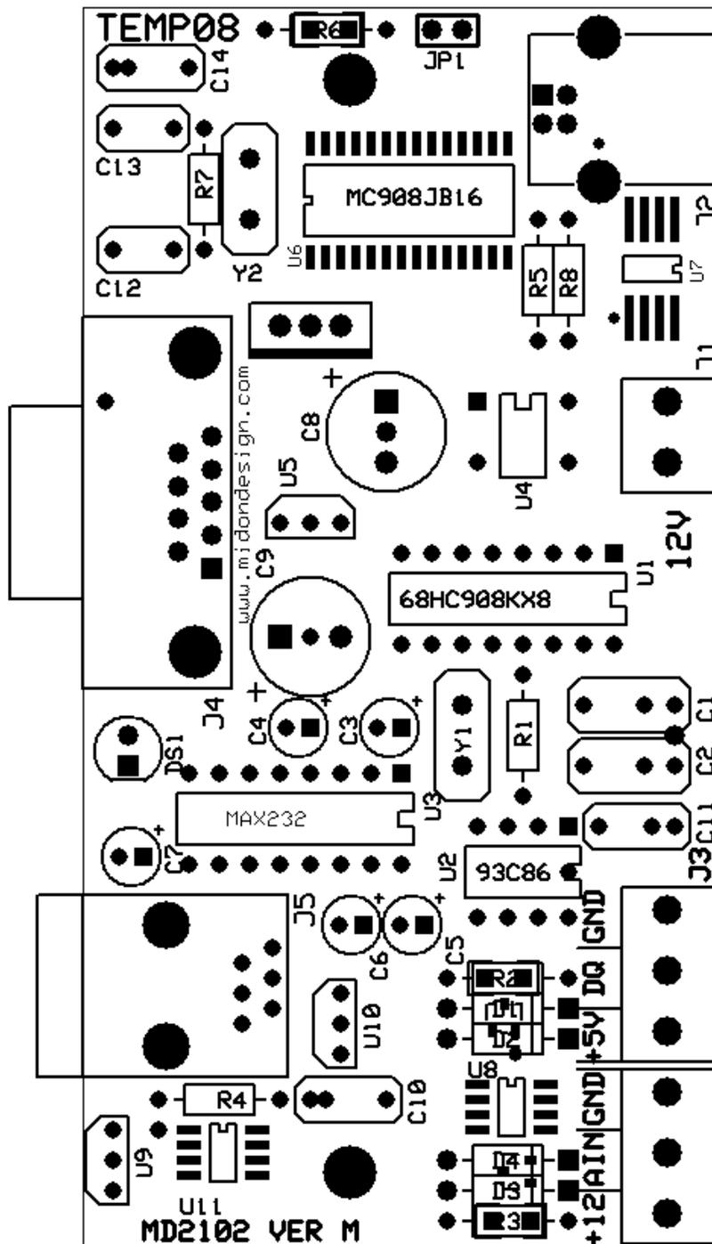
Figure 3 TEMP08 Parts Placement
